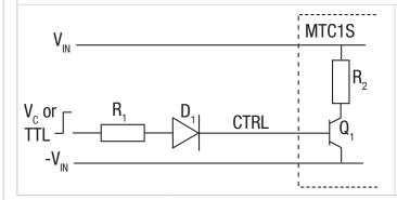
$\rm D_1(e.g.~1N4001)$  is necessary for correct operation of the MTC1 when the control signal is LOW. The recommended drive current  $\rm I_g$  to shut down the MTC1 is 6mA to 15mA. The value of R, can be derived as follows:
