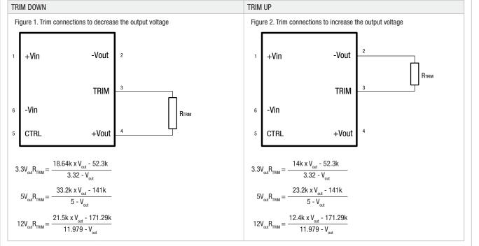
Accuracy of adjustment is subject to tolerances of resistors and factory adjusted output accuracy. Vout is equal to the desired output voltage.
